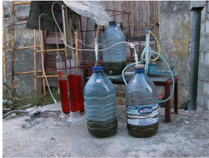
FIGURE 1. Biodigester (reduced model) and micro gauge utilized.
