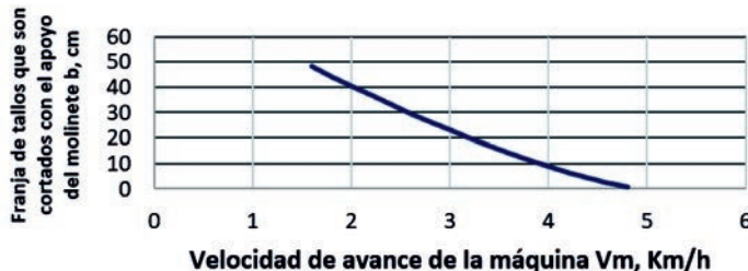
FIGURE 7. Influence of the Speed of Advance of the Machine on the Strip of Stems that are Cut with the Reel Support, for a Reel Radius R_m = 47 cm, a Number of Blades Z = 5 , a Reel Rotation Speed \omega = 8 rpm and an Output of the Reel c = 15 cm.
