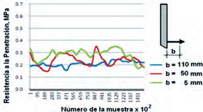
FIGURE 4. Continuous recording of the soil strength penetration with prismatic probes 30° x 520. H_m = 29,10\% ; \gamma_m = 0,95 \text{ g}\cdot\text{cm}^{-3} ; V_{m2} = 0,867 \text{ m}\cdot\text{s}^{-1} . FIGURA 4. Registro continuo de la resistencia a la penetración con sondas prismáticas 30° x 520. H_m = 29,10\% ; \gamma_m = 0,95 \text{ g}\cdot\text{cm}^{-3} ; V_{m2} = 0,867 \text{ m}\cdot\text{s}^{-1} .
