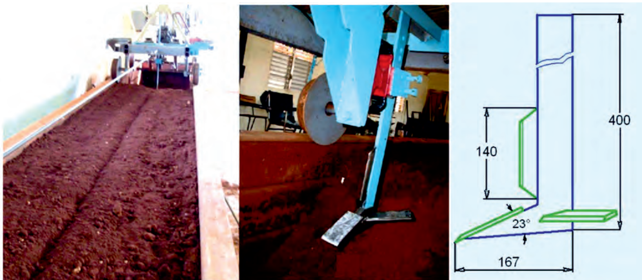
FIGURE 1. Trolley over railway (a), tool transducer (b) and tool dimensions (c).
