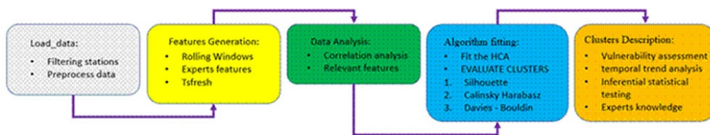
Figure 1. Pipeline of process for clustering time series
