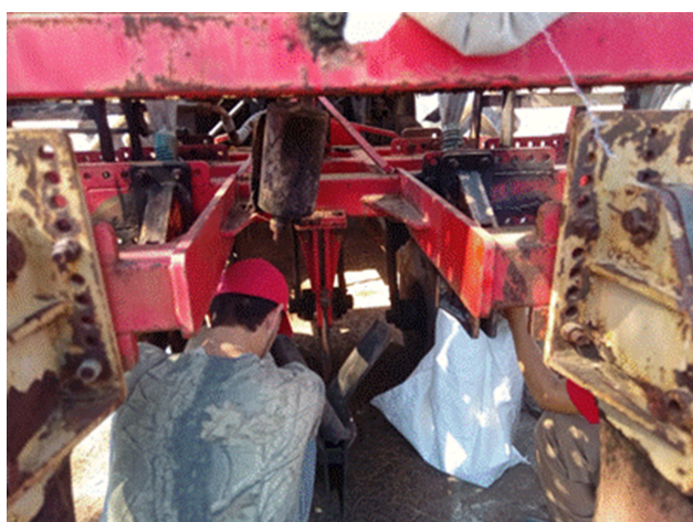
Figure 1. Positioning of the bags in the discharge tubes of the fertilizer spreader FMCM-1.
