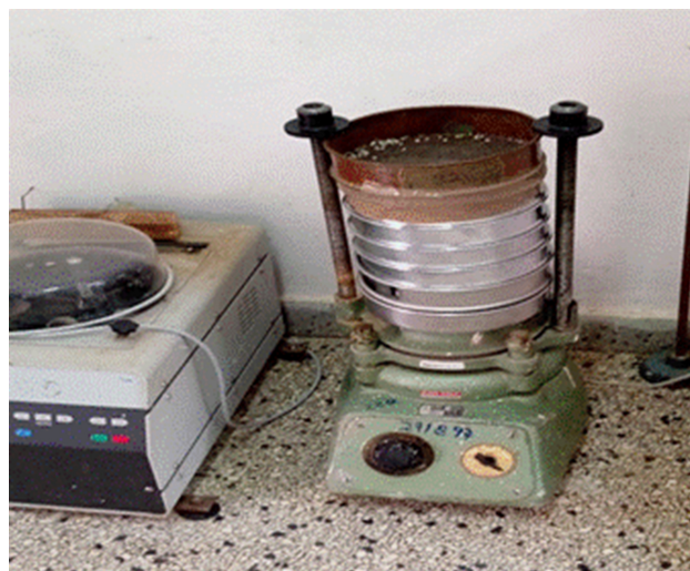
Figure 1. Sieve vibrator used for determining particle size distribution.
