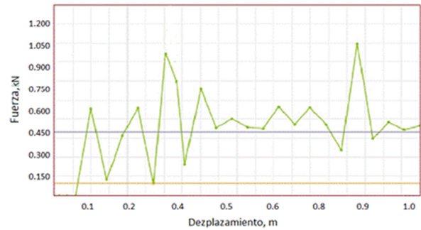
FIGURE 5. Draft force versus displacement.
