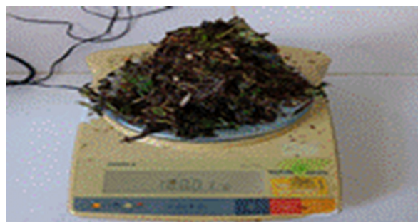
FIGURE 2. Electronic scale model LG-1001 from 0 to 1000 (g)/0.1 (g).
