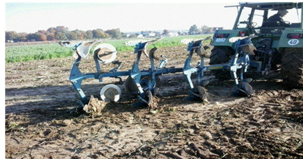
FIGURE 2. Reversible moldboard plow with 4 working organs during ploughing. Source: Author's file.
