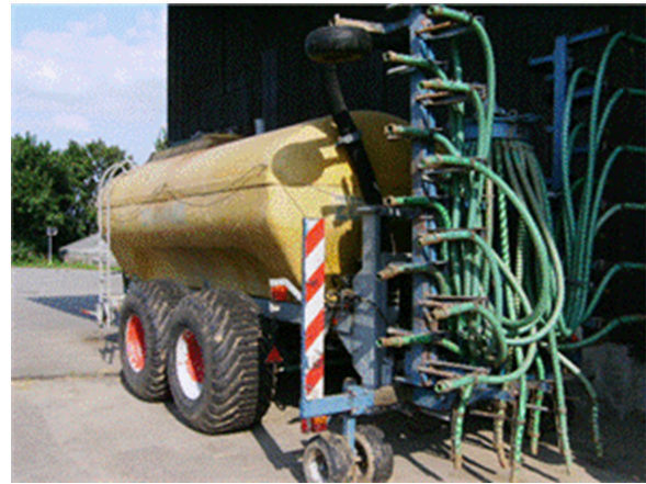
FIGURE 8. Liquid organic fertilizer spreader (effluent). Source: Author's file.
