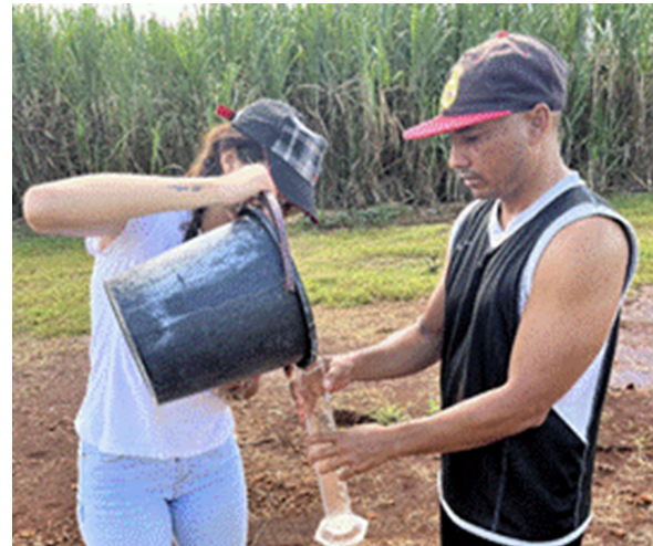
FIGURE 3. Volumetric capacity of the sprinklers.
