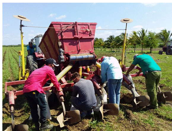
FIGURE 2. Obtaining the delivery of organic mineral fertilizer Agromena - G for each one of the outputs of the fertilizer spreader.
