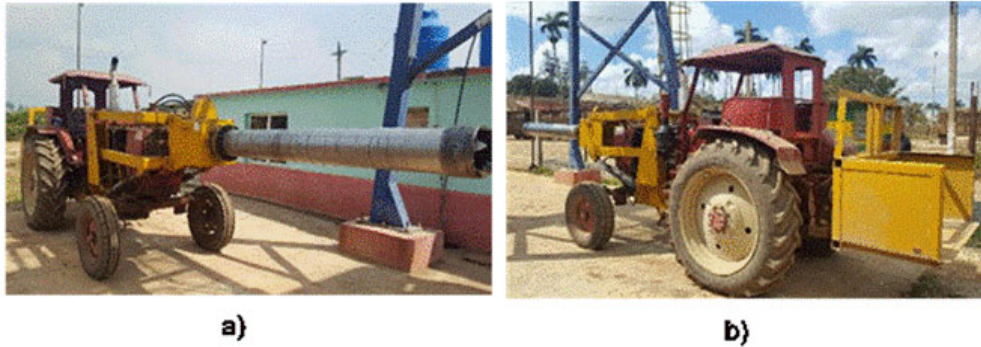
FIGURE 1. Sampling probe (a) and basket (b) coupled to the Yum-6 tractor.
