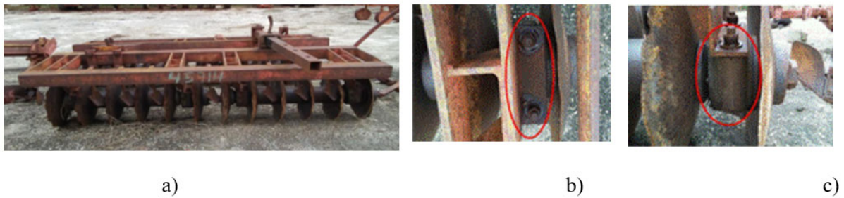
FIGURE 2. Location of bearing support body on harrow of 4500 lb.; a) Harrow elements set, b) Top view and c) Side view.
