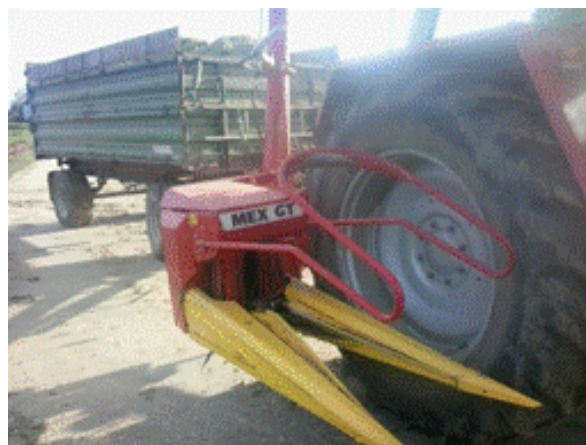
FIGURE 1. Silo cropper of small format working.
