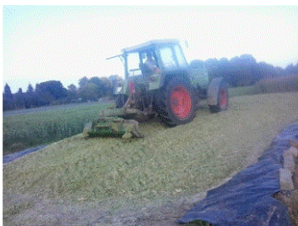
FIGURE 3. Compacting of the forage in soil silo of small format. Source: Author's file.
