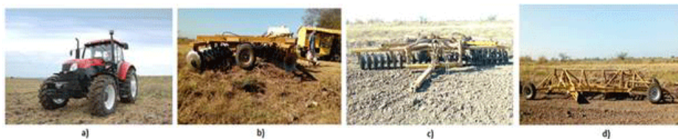
FIGURE 1. Tractor used to form aggregate with harrows and land plane. a) Tractor YTO x1204. b) Medium Baldan harrow with 40 discs. c) Baldan heavy harrow with 52 discs and d) Land plane of national manufacture.
