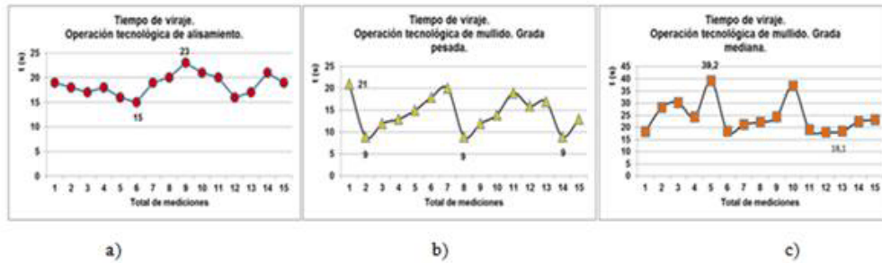
FIGURE 2. Turning time a) YTO X 1204 tractor and Holmeca land plane. b) YTO X 1204 tractor and the 52-disc heavy harrow. c) YTO X 1204 tractor and the medium 40-disc harrow.
