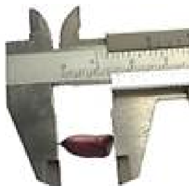
FIGURE 2. Determination of peanut kernel length.
