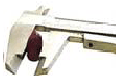
FIGURE 3. Determination of the equatorial diameter of the peanut kernels.
