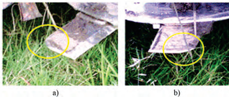
FIGURE 9. Wear at the rounded ends: a) Due to inadequate cutting height; b) Due to inadequate angulation.
