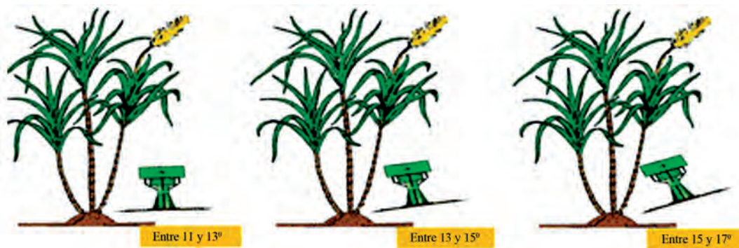
FIGURE 8. Recommended magnitudes of the base-cutter angles (Abadia, 2018).
