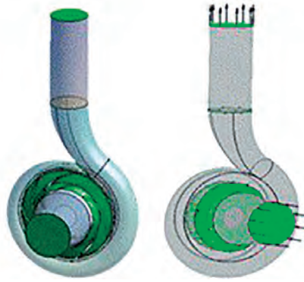
FIGURE 6. Zones in which the system boundary conditions were located for the simulation of the single suction centrifugal pump model BSC 80/200 (130-65). FIGURA 6. Zonas en las que se ubicaron las condiciones de contorno del sistema para la simulación de la bomba centrífuga de simple succión modelo BSC 80/200 (130-65).
