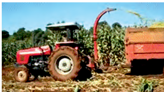
FIGURE 1. Unit consisting of the MF 275 tractor and the KUHN MC 90S TWIN combine harvester. FIGURA 1. Conjunto formado por el tractor MF 275 y la cosechadora KUHN MC 90S TWIN.
