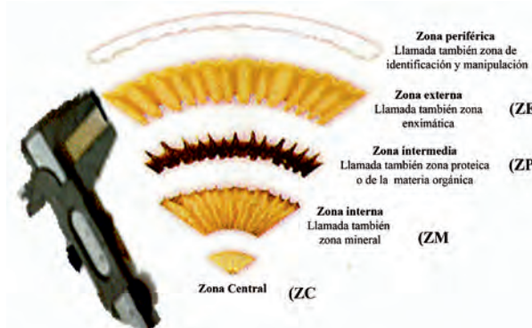
FIGURE 1. Zones that make up the chromatogram. FIGURA 1. Zonas que componen el cromatograma.
