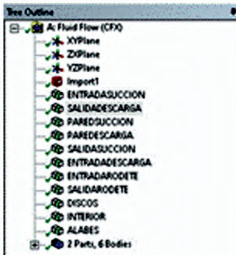
FIGURE 4. Faces that are declared to locate the boundary conditions. FIGURA 4. Caras que se declaran para ubicar las condiciones de contorno.
