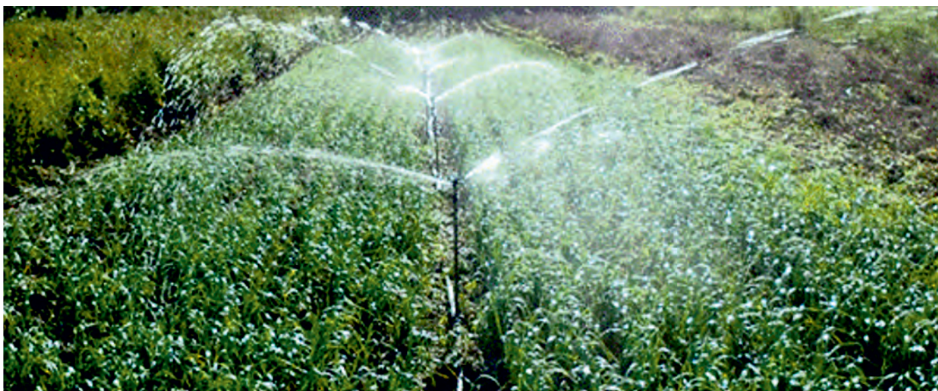
FIGURE 2. Irrigation side with sprinklers operating simultaneously. FIGURA 2. Lateral de riego con los aspersores funcionando simultáneamente.
