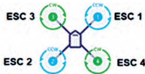
FIGURE 11. Engine Number and Direction of Rotation. FIGURA 11. Numero de motor y sentido de giro. Source: GyuJin et al. , 2020.
