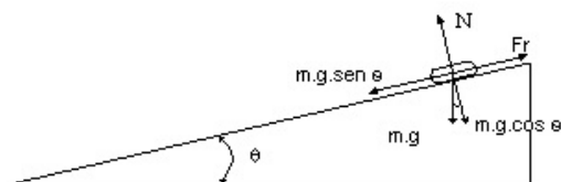
FIGURE 1. Apparatus and free body for the determination of friction coefficient. Source: file of the author.
