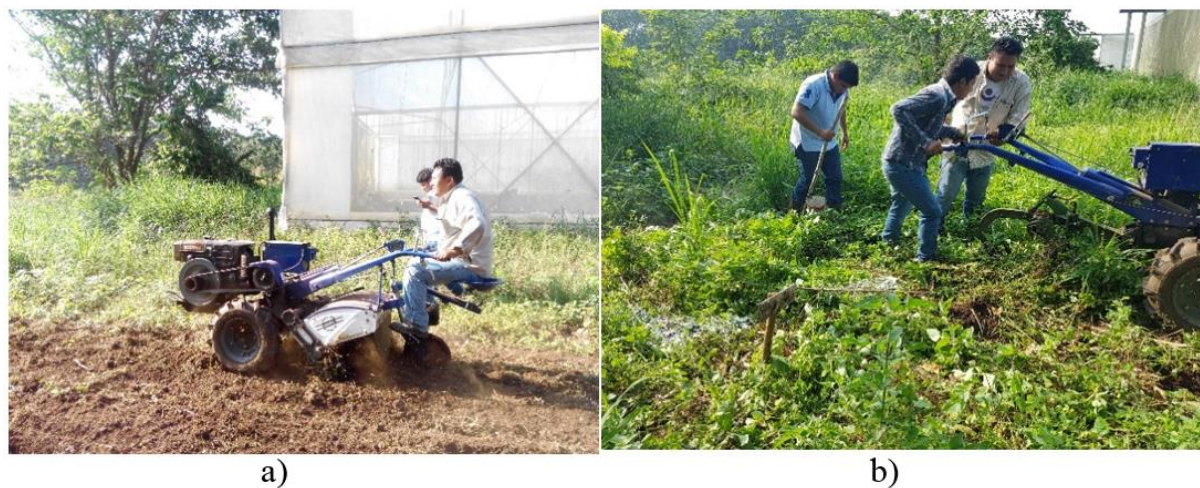
FIGURE 2. Implement-tools in the test, a) cultivator and b) plow.
