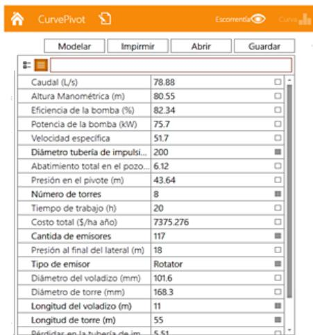
**FIGURE 8.** Results screen of the irrigation system.
