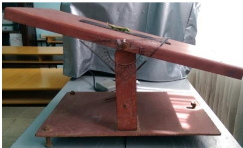
FIGURE 5. Determination of the angle of friction for sheaths in the inclined plane.
