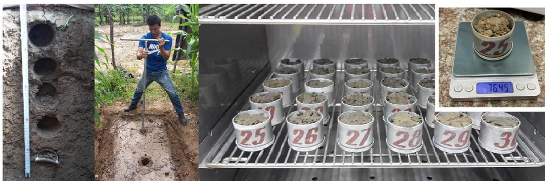
**FIGURE 2.** Sample extraction and processing in the laboratory for the determination of field capacity, real density, bulk density and porosity.
