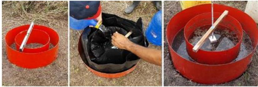
**FIGURE 3.** Placement of the Infiltration Rings for the determination of water infiltration rate at one of the observation points.
