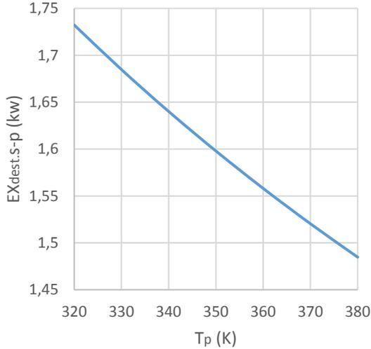
**FIGURE 11.** Variation of the exergy destroyed in the sun-plate transference versus the temperature of the plate.
