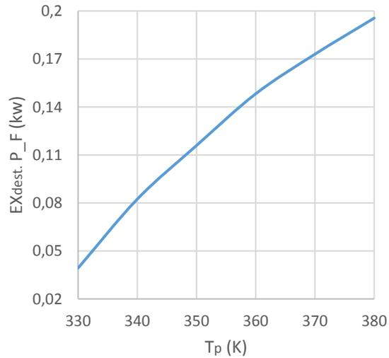
**FIGURE 12.** Variation of the exergy destroyed in the plate- heat fluid heat transference versus the temperature of plate.
