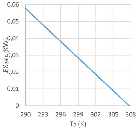
**FIGURE 6.** Variation of the exergy gained by the work fluid versus the ambient temperature.
