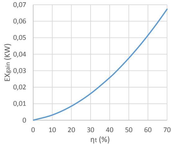
**FIGURE 3.** Variation of the exergy gained by the fluid versus the energetic efficiency of the collector.
