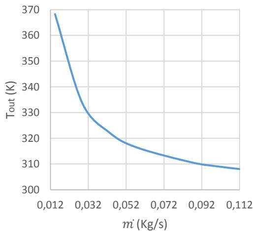
**FIGURE 8.** Variation of the temperature of the fluid outlet versus the variation of the mass flow rate.
