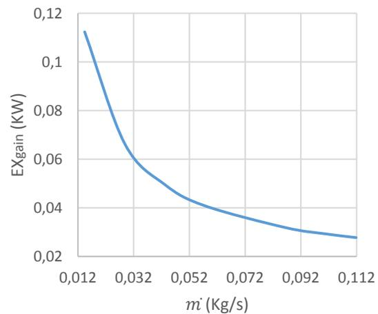
**FIGURE 9.** Variation of the exergy gained by the fluid versus the variation of the mass flow rate.
