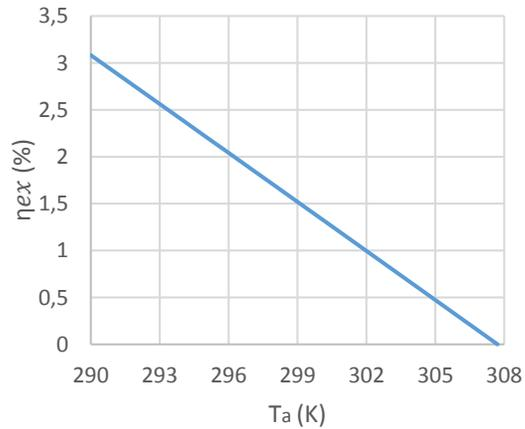
**FIGURE 7.** Variation of the exergetic efficiency of the collector versus the ambient temperature.
