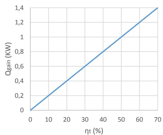
**FIGURE 5.** Variation of the heat gained by the work fluid versus the energetic efficiency of the collector.
