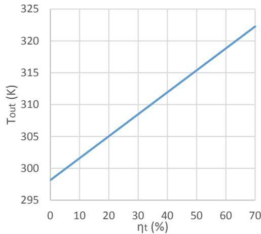
**FIGURE 2.** Variation of the temperature of the fluid outlet versus the energetic efficiency of the collector.
