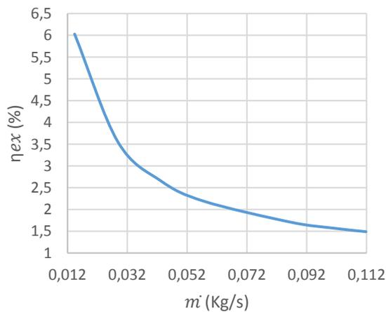
**FIGURE 10.** Variation of the exergetic efficiency of the collector versus the variation of the mass flow rate.
