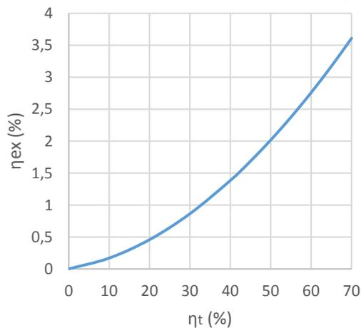
**FIGURE 4.** Variation of the exergetic efficiency versus the energetic efficiency of the collector.
